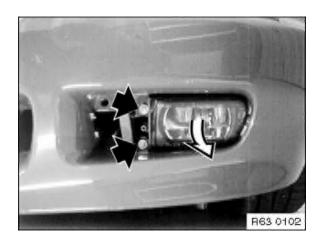
Unfasten screws, pry out headlight insert and remove connector.
